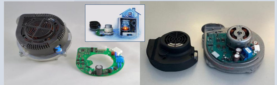
ECU CONTROL UNIT FOR BRUSHLESS MOTOR CONTROL IN CONDENSING BOILERS (HOME APPLIANCES)
