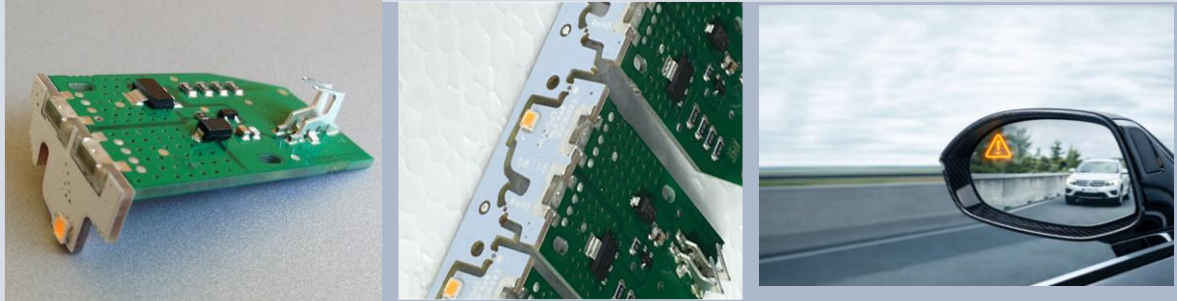
ELECTRONICS FOR SMALL LIGHTING DEVICES: TURN SIGNALS, SIDE MARKER WARNING LIGHTS, COURTESY LIGHTS, REFLECTORS (AUTOMOTIVE)
